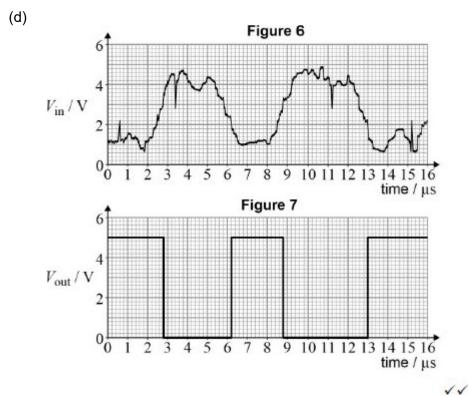
1st mark - 0 to 5 V sq wave with 3 marks and two spaces
