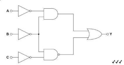
**MP1**: all inputs inverted (accept a shorted-out NAND or NOR gates for the inverters)
