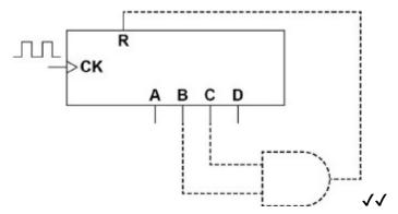
1 mark for use of the correct counter outputs 1 mark for the correct logic gate connected to reset **R**
